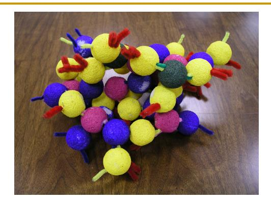
Yellow balls represent Te atoms and red sticks represent their lone-pairs. The dark balls are Ge, Si and As. The coordination can vary from site to site, however, in the model we have shown Ge and Si as 4-coordinated and As as 3-coordinated.
