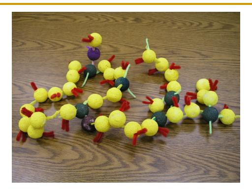
Yellow balls represent Te atoms and dark sticks represent their lone pairs. Dark balls are Ge atoms. The purple ball is Sb. To fit particular device needs other elements can be added.
